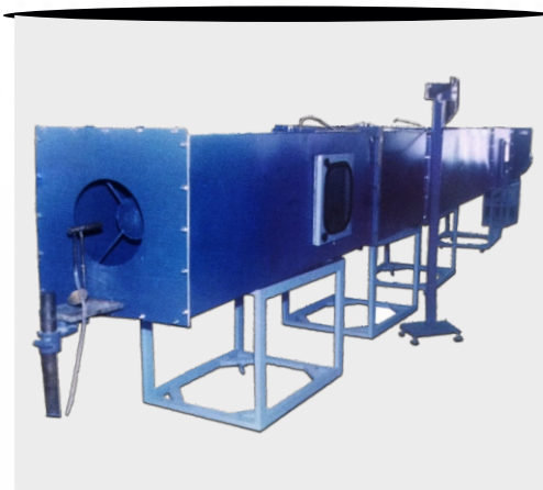
Test - Rig as per B.S. 6540
