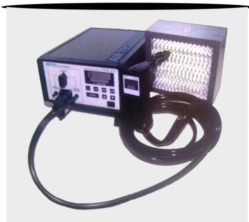
Photo meter For Testing of HEPA Filter
