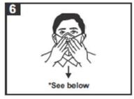
\*6. To check fit, place both hands completely over the mask and inhale. If air leaks around nose, readjust the nose clip. If air leaks at the mask edges, work the straps back along the sides of your head. Repeat the procedure until respirator is sealed properly.
