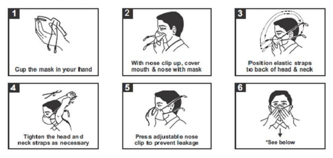
\*6. To check fit, place both hands completely over the mask and inhale. If air leaks around nose, readjust the nose clip. If air leaks at the mask edges, work the straps back along the sides of your head. Repeat the procedure until respirator is sealed properly.
