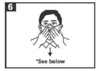
\*6. To check fit, place both hands completely over the mask and inhale. If air leaks around nose, readjust the nose clip. If air leaks at the mask edges, work the straps back along the sides of your head. Repeat the procedure until respirator is sealed properly.
