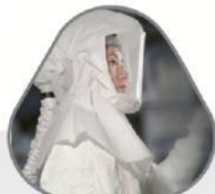
Positive Pressure Respirator: Constant Flow Type- Air hood is loose fitting face piece which cover the entire head-inlet air pressure must be able 6 cfm ( Cubic Feet per Minute for a loose-fitting hood.
