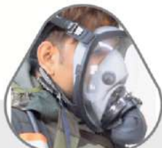
Positive Pressure Respirator: Constant Flow Type- Full facepiece maintain a slight positive pressure of air inside the facepiece whether the wearer is inhaling or exhaling. This helps prevent contaminants from seeping around the facepiece, even if there should be small breaks in the face-to-facepiece seal. Inlet air pressure must be able to maintain at least 4 cfm ( Cubic Feet per Minute for a tight-fitting face piece
